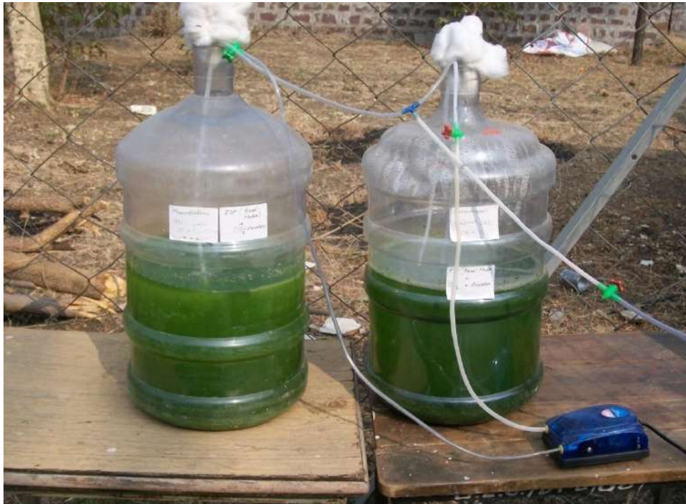
Microalgae Cultivation by using Carbon Dioxide and Aeration in Energy Park RGPV Bhopal
