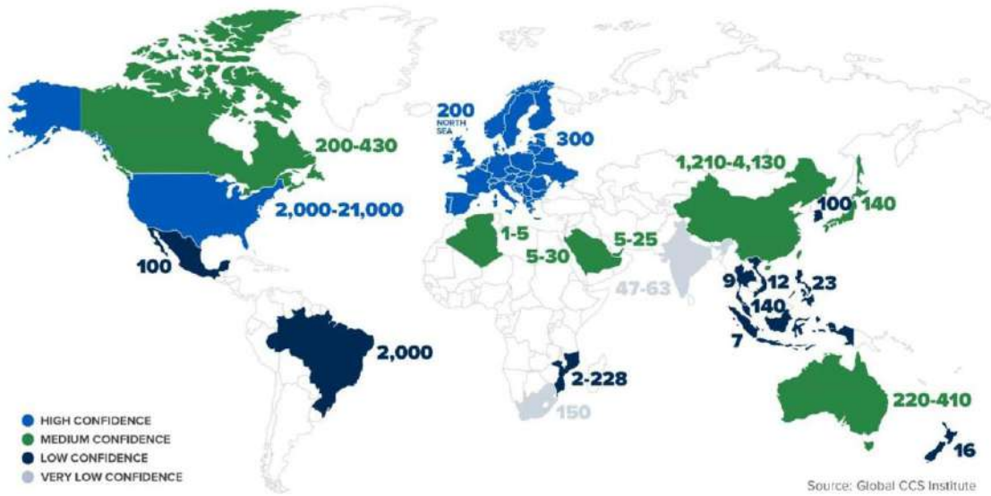
Figure 2: Estimated CO 2 Geological storage capacity – billions of tonnes.
