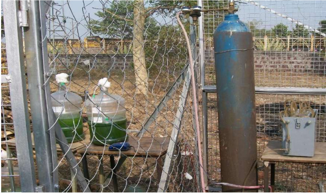
Microalgae Cultivation by using Carbon Dioxide and Aeration in Energy Park RGPV Bhopal
